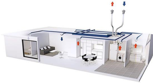
Figure 9. Whole apartment balanced heat recovery using air to air heat pump unit. Source: Nilan.
